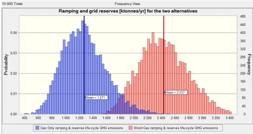
**Figure 4.** Changes in life-cycle GHG emissions [ktonnes] related to grid reserve and gas turbine ramping for the two alternatives.
