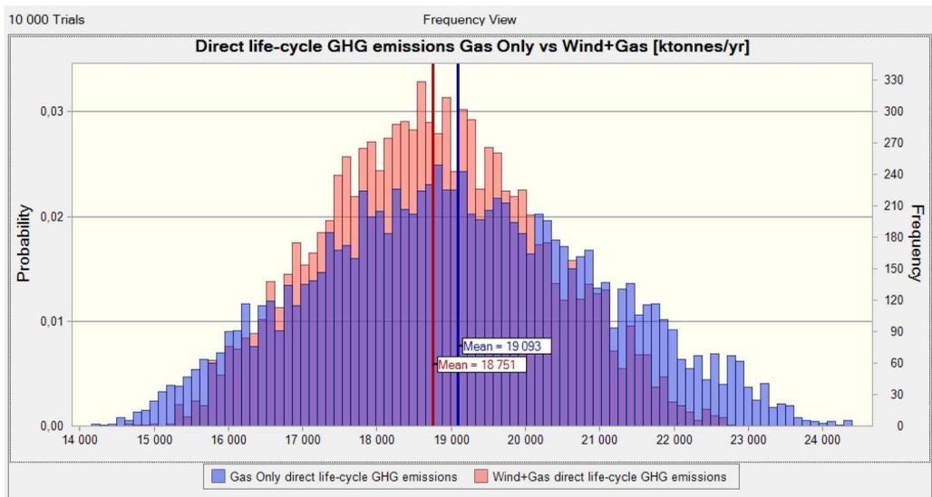
**Figure 5.** Direct life-cycle GHG emissions [ktonnes/year] of the Irish grid for both alternatives.
